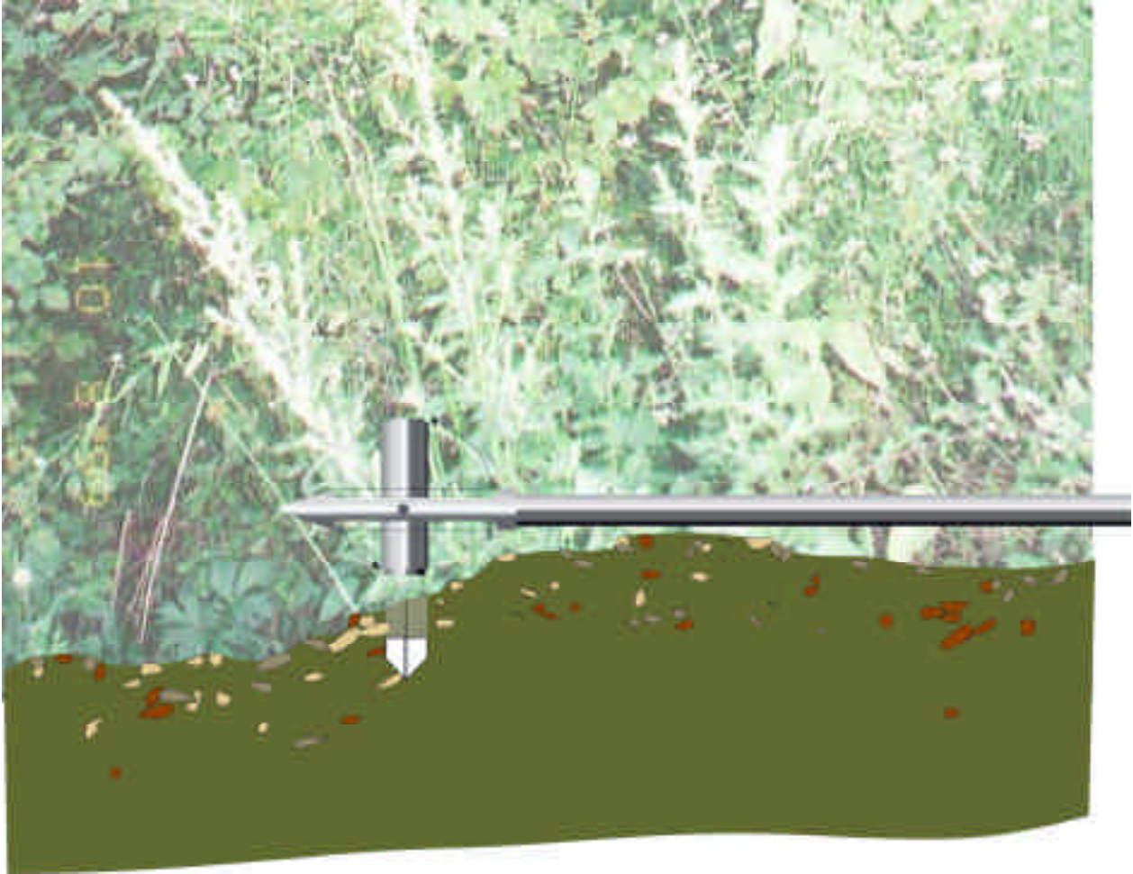
Figure 4: Concept drawing of target insertion tool. The tool is inserted through scrub and vegetation from a safe area up to 6 metres away. On remote activation, the target insertion "gun" rotates to a vertical position (shown) and injects a target into the ground beneath it, to a prescribed depth.
