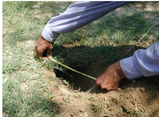
Figure 2 Measuring hole left by deminer after metal detection and prodding to remove metal fragment
